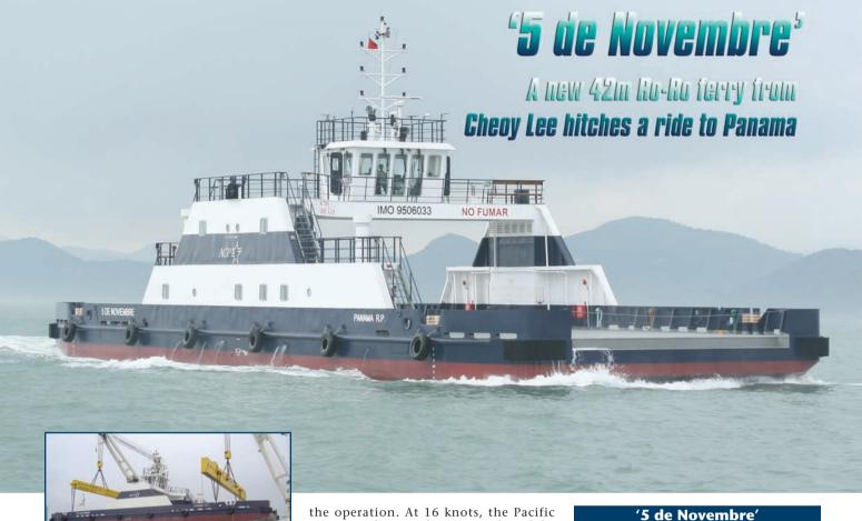
Unlike the recent series of eight Cheoy Lee-built Z-tech 6000 tugs for the Panama Canal Authority that have made the 10,000nm Pacific crossing from Hong Kong to Panama, this open-bowed, flat-bottomed vessel, powered by only a pair of 298kW Caterpillar diesels, required transportation aboard a larger vessel.
