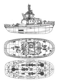
With significant separation between the two forward thrusters and single aft drive unit, the thruster setup greatly enhances vessel manoeuvrability, allowing the vessel to operate effectively in confined spaces at all speeds, said Cheoy Lee. Other benefits of the Rotortug arrangement includes enhanced safety during towing and escort operations, added levels of redundancy, and a higher bollard pull in all directions.
